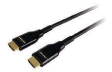
CRS-PLUGNVIEW-H cable is a high-speed HDMI active optical cable (AOC) designed with heavy-duty durability perfectly suited for the harshest use and abuse expected from rental and road applications. CRS-PlugNView-H supports resolutions up to 4K@60 (4:4:4) 18 Gbps over long cable runs up to 100 meters without the need for an external power supply or additional extenders.
