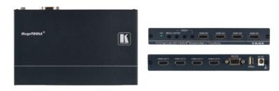
VA-4X is a versatile 4K@60Hz (4:4:4) HDMI multi-channel extender that equalizes and reclocks TMDS data before re-transmitting the signal, thus increasing the HDMI cable range for all 4 outputs. It is a true 4-channel HDMI "Toolbox", with functionality including 4 independent test-pattern generators, chroma sub-sampling down-conversion and EDID management options.
