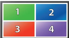
**QUAD-MODE:** In Quad mode, the screen is split into four fields of equal size with the four video sources or computers being displayed in each of these fields. Keyboard and mouse operation can be assigned to the field of the corresponding computer.
