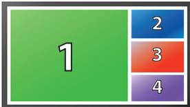
**PiP MODE:** In the PiP (picture in picture) mode, the full screen displays of one of the four video sources, and is accompanied by three smaller images (thumbnails) containing the other video sources on the right-hand margin of the screen, allowing simultaneous monitoring.
