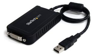
The USB2DVIE3 USB DVI Video Adapter offers a perfect external multi-monitor solution, enabling you to add a high-resolution (up to 1920x1200) external DVI output to your desktop or laptop computer system using an available USB 2.0 port.
