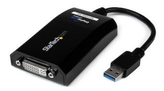
The USB32DVIPRO USB 3.0 to DVI Adapter turns an available USB 3.0 port into a DVI output, with high resolution 2048x1152 video support - a convenient external video solution that makes it easy to add multi-monitor capability to a USB 3.0-enabled desktop or laptop computer (optimal performance from USB 3.0, backward compatible with USB 2.0).
