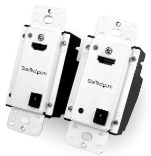
The ST121HDWP HDMI over CAT5 Extender Wall Plate Kit lets you extend your HDMI audio/video up to 165 feet (50 meters) over Cat5e or Cat6 cabling. For a seamless, professional installation, you can install the included transmitter and receiver units into wall plates, with the added versatility of Power Over Cable enabling both units to be powered by the same single power source.
