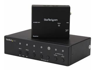
This multi-input video extender kit uses HDBaseT technology to extend your video signals up to 230 feet (70 meters) over a single CAT5e or CAT6 cable. It features a built-in video switch that enables you to choose which video source is outputted from four independent video sources (2 x HDMI, 1 x VGA and 1 x DisplayPort). The video extender supports Ultra HD 4K and Full HD 1080p video resolutions, with support for the accompanying digital 7.1 audio.
